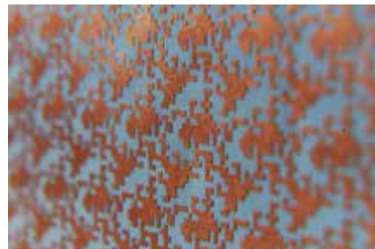
■ Genetically optimized metasurface for wideband polarization conversion
